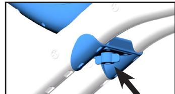
2. Turn both legs of the frame 180° to the other side. You will notice that the frame legs hinge around the handlebar.
