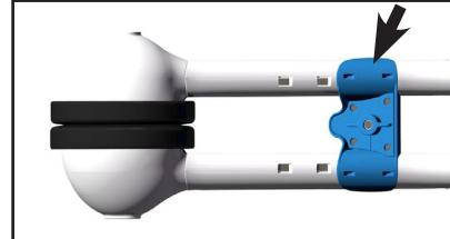
**ATTENTION: NOTE THAT IN 3-WHEEL POSITION ONLY THE LOWEST SEAT POSITION IS AVAILABLE AND IN 2-WHEEL POSITION ONLY THE HIGHEST SEAT POSITION IS AVAILABLE. DO NOT ATTEMPT TO FIT THE SEAT AT THE HIGH POSITION IN 3-WHEEL MODE OR AT THE LOW POSITION IN 2-WHEEL MODE. ALWAYS MAKE SURE THE FITTER STUBS FIT IN THE FITTER HOLES IN THE BOTTOM OF THE FRAME TO ENSURE A GOOD SEAT FIXATION.**
