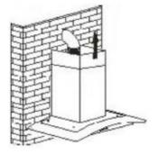
Slide the top part of the chimney inside the bottom and pull the top up to the desired height.
